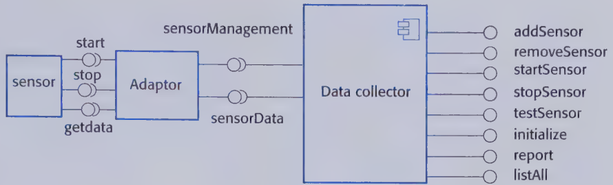
Figure 16.12 An adaptor linking a data collector and a sensor
